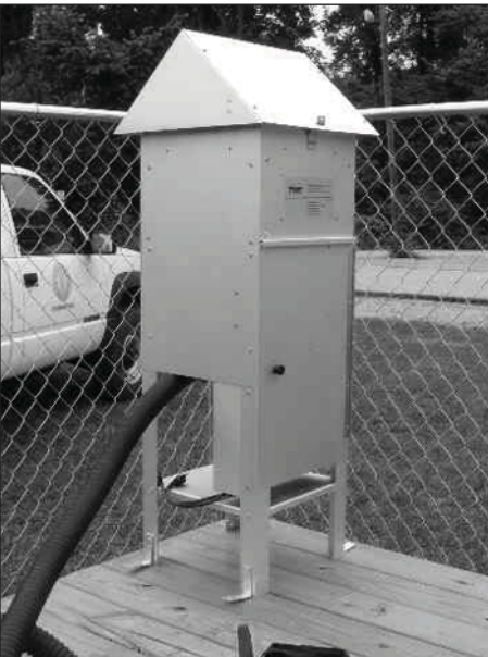
This monitor records air samples to determine if hazardous air pollutants are present. Division for Air Quality photo
